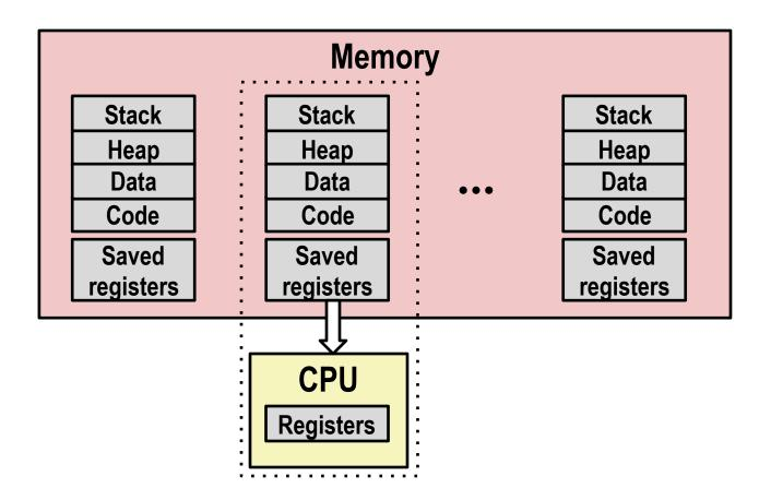
Load saved registers and switch address space (context switch)
