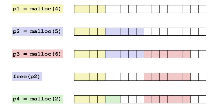
(Arguments to malloc are in words for simplification, i.e. malloc(4) allocates 4 words.)
